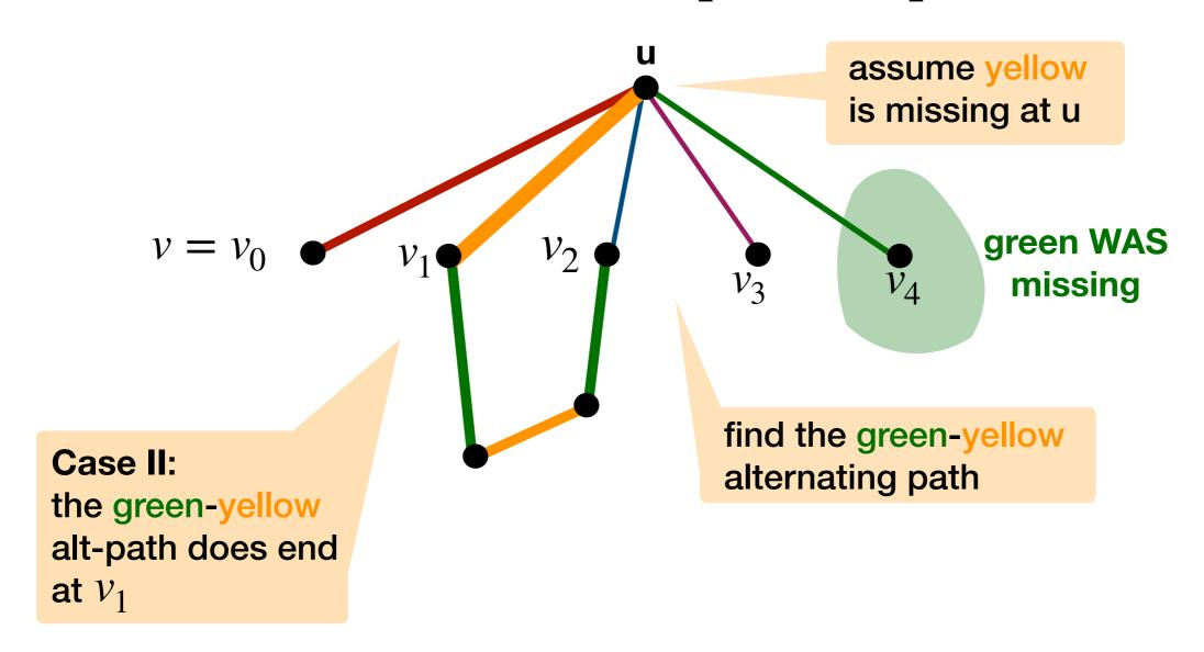
Two bottlenecks in maintaining a  $\Delta + 1$  coloring
